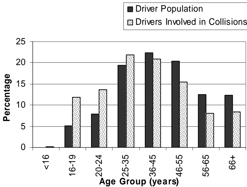
Figure 11: Percentage of licensed drivers, and licensed drivers in injury or fatal collisions, by age group, BC, 2002. (ICBC, 2002)
